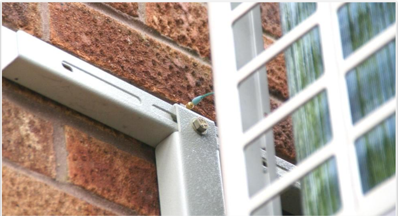
Picture 5-2. 486 Stroud, Wall-mounted Accelerometer
