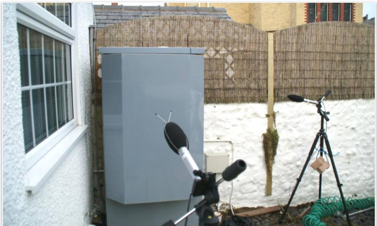
Picture 5-7. 440 Fylde, ASHP and Microphone Arrangement
