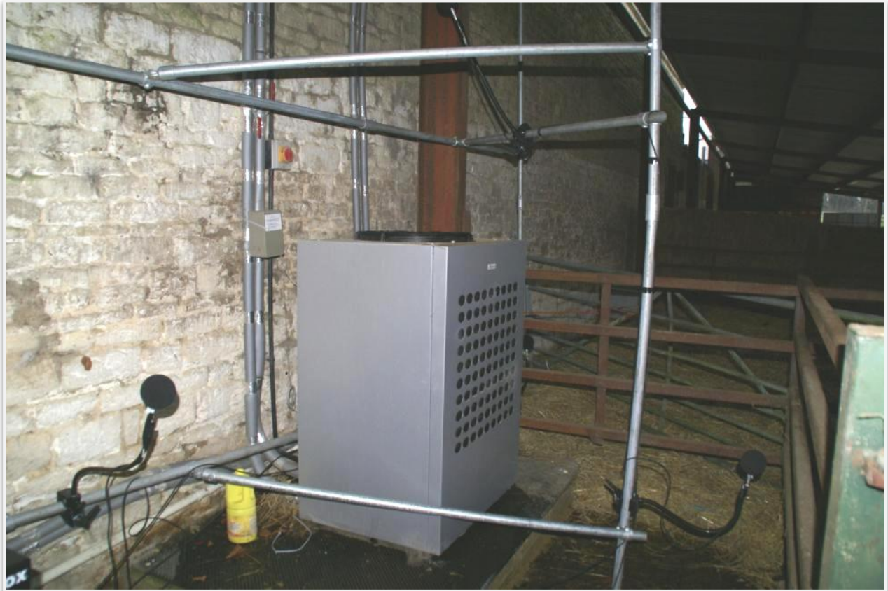
Picture 5-25. 479 Cotswold (Stables), ASHP and Microphone Arrangement
