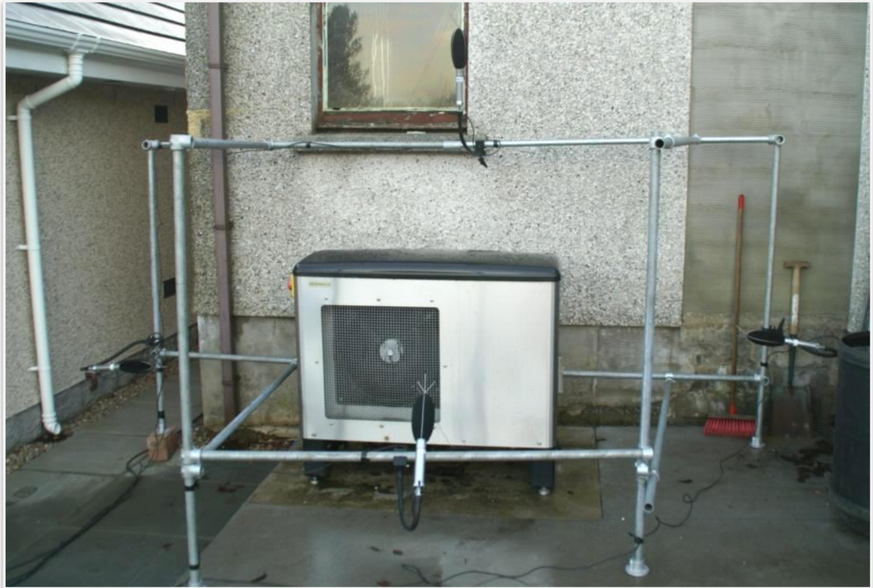
Picture 5-9. 418 Central Buchan, ASHP and Microphone Arrangement
