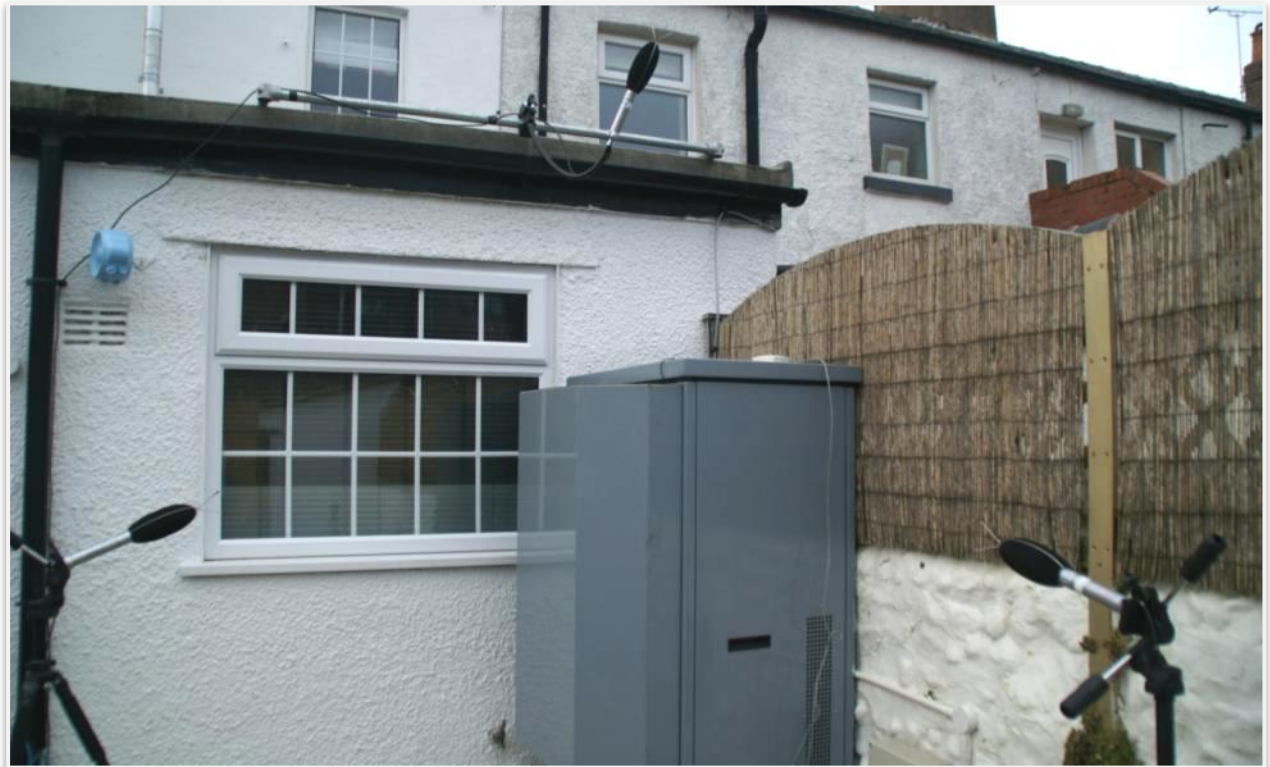
Picture 5-6. 440 Fylde, ASHP and Microphone Arrangement
