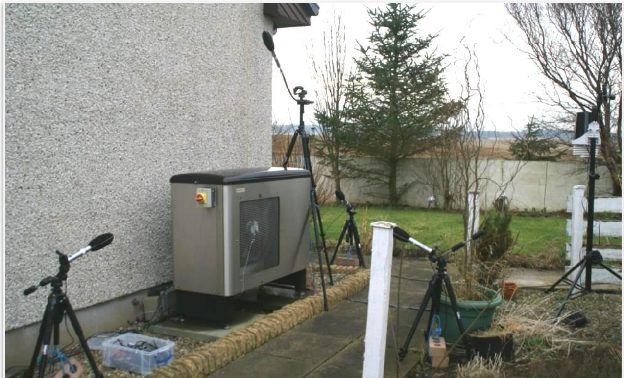
Picture 5-11. 422 Fraserburgh, Original ASHP and Microphone Arrangement
