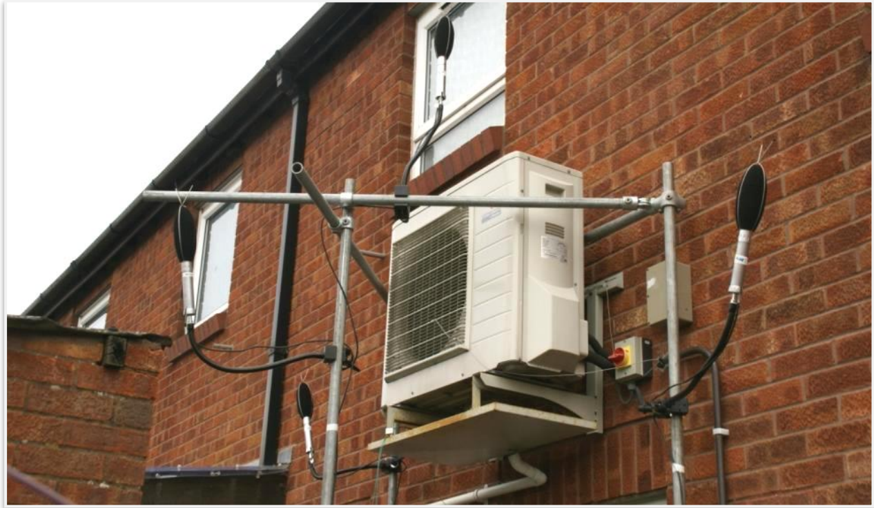
Picture 5-3. 486 Stroud, ASHP and Microphone Arrangement
